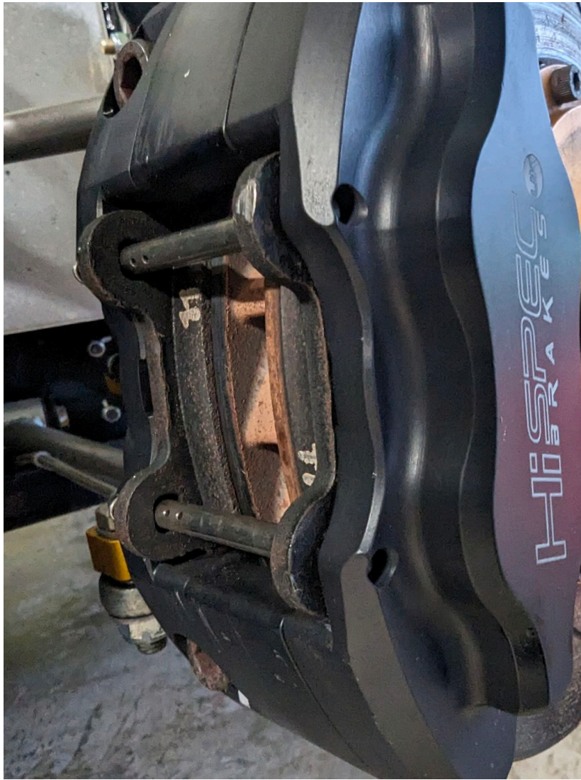
Figure 26: Shaved brake pads to clear Braid wheels (see top right of bracket)
