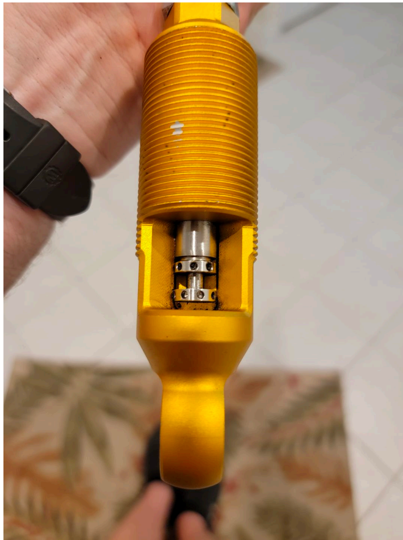
Figure 20: An opened shock. The top adjuster is rebound, the bottom is compression. Turn right to close, left to open.
