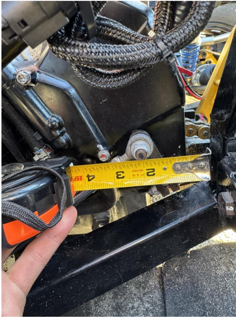
Figure 16: Distance between the shifter bolt (at the 2" mark) to the case bolt on the left with a red mark should be 1.25".
