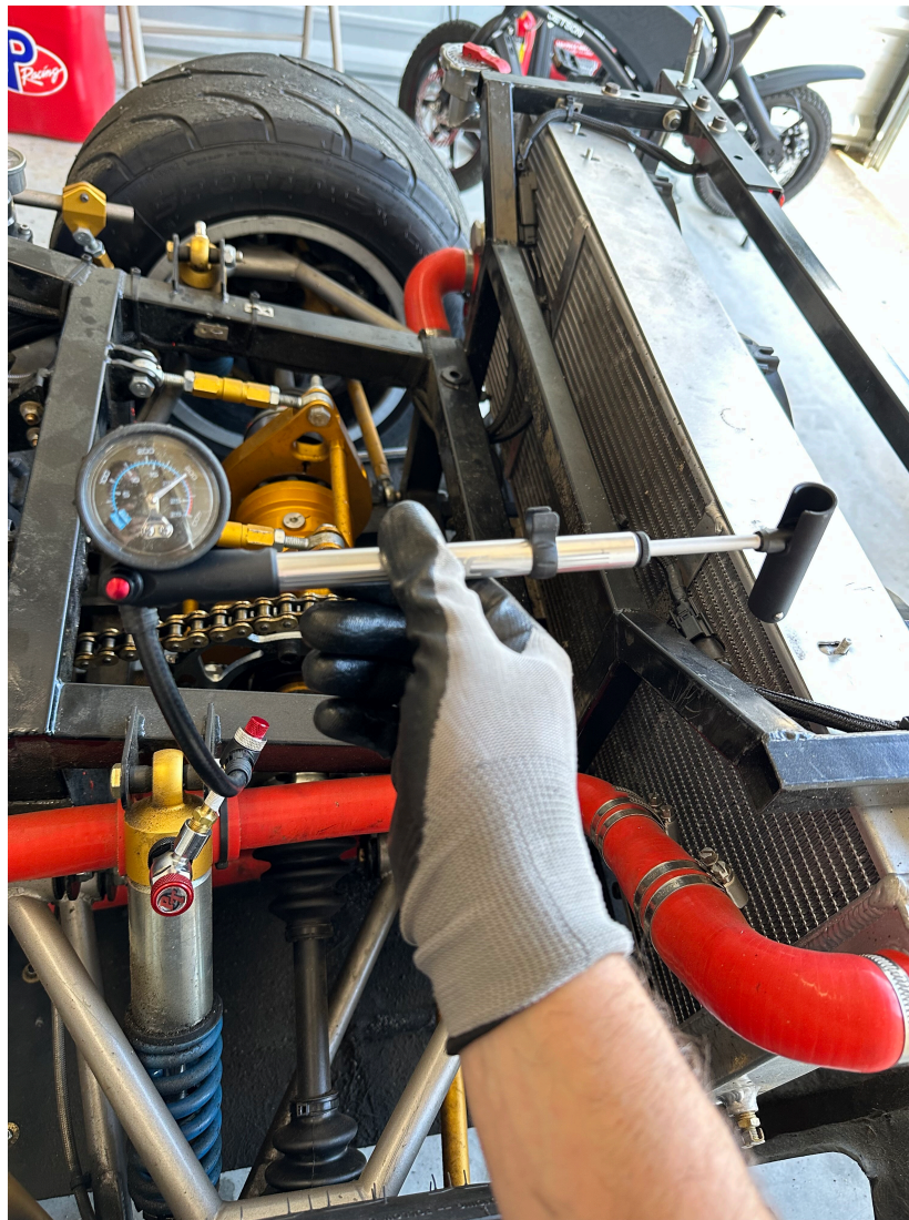
Figure 9: Checking shocks at 300psi with Amazon pump. The no-loss chuck is not necessary with this pump and was later removed.
