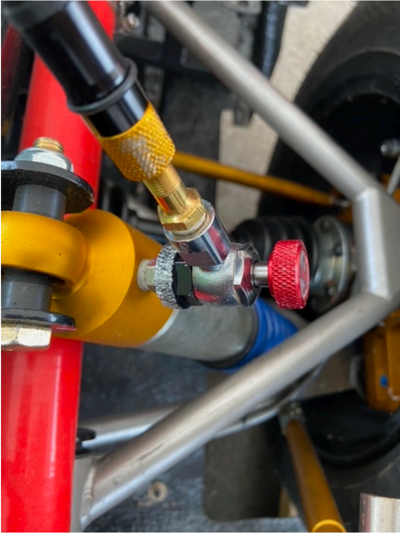
Figure 8: Checking pressure with no-loss chuck.
